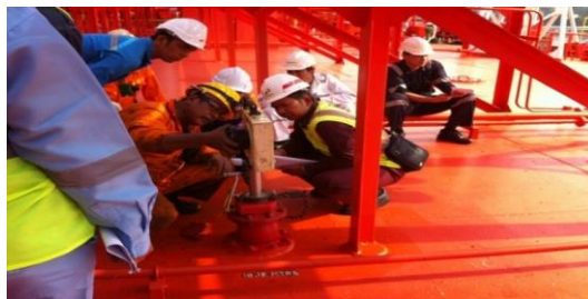
Figure 4. Tank sounding on the MT ship. Nirbita
